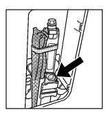
Remove the wing-bolt on the jack and then remove it.
